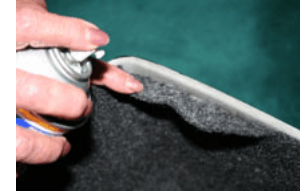
12. Check your edges for loose lining. Add adhesive where required.
