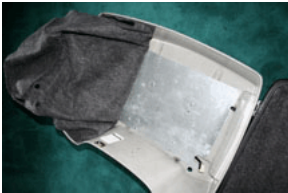
10. Once this panel is in place, fold back lining to expose the box.
