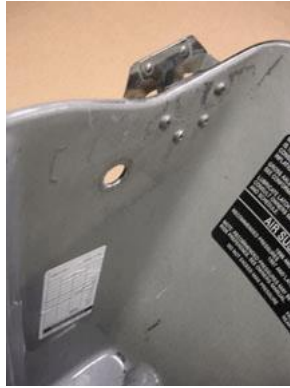
2: Remove rubber grommets but leave bracket on.
