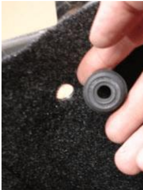
4: Position lining in bag and install grommets.
