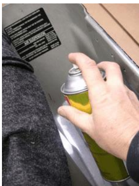
7: Spray adhesive on the floor, 2 ends and the one free side. Spray the adhesive liberally...as pictured! (This will allow you to easily move your lining into position.)
