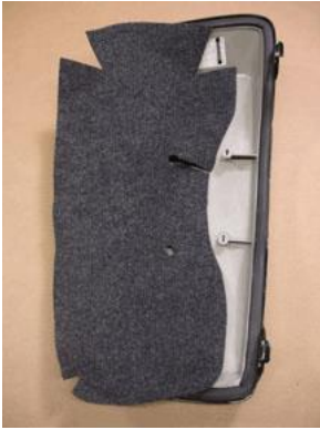
1: Place lining into lid for fitment.
