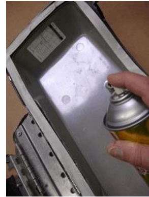
3: If you are leaving the seal on, mask it! Spray the lid with plenty of adhesive!
