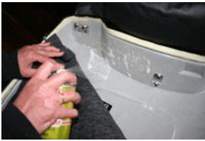
4. Mask around gasket seal to prevent adhesive over spray. Pull back liner and spray adhesive liberally... lots. It lets the lining slide around easily into place.
