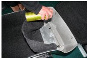
11. Spray & work your way around the box pushing lining into place.
