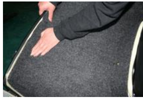
5. Push lid liner into position working your way around the lid. Spray one panel at a time.
