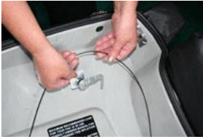
1. Remove wire stay and lock in the lid. Clean inside surfaces.
