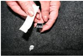
7. After smoothing out the seams in the box liner, locate the lighting cord, run it through the hole and mask it.
