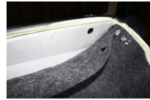
6. Now spray the last side panel after removing the lock. Once completed reinstall lock into place.
