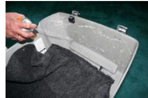
9. Start with this side panel. Spray adhesive liberally and push liner into place. Work out wrinkles with your hand.
