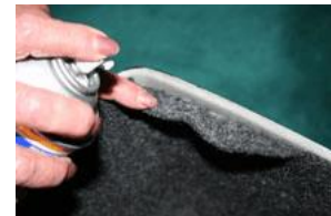
12. Check your edges for loose lining. Add adhesive where required.
